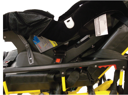
Figure 31 – Secure the waist restraint
